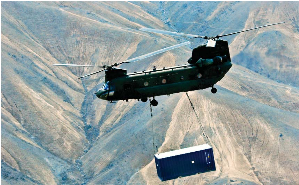
A U.S. Army CH-47 Chinook helicopter carries a sling-loaded shipping container in Afghanistan. It has been reported that India is planning to 15 Chinook heavy-lift helicopters at estimated cost of around $1 billion. 21
